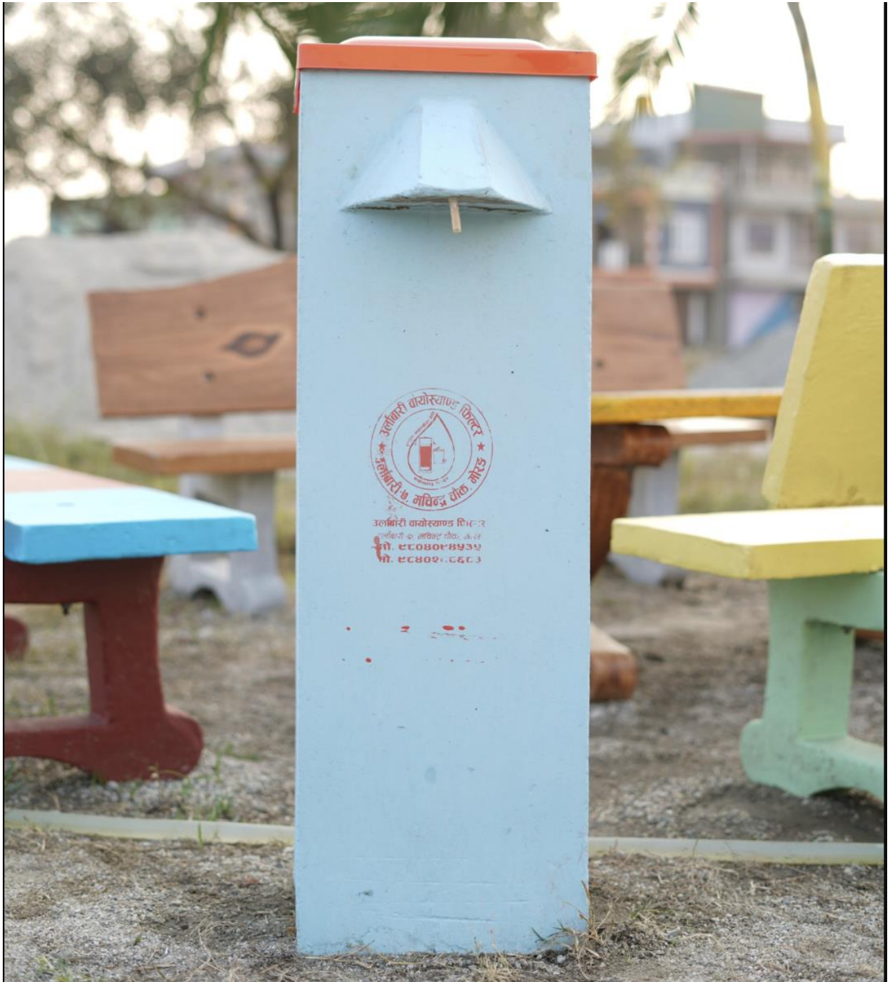
FIGURE 1 : BIO SAND FILTER
